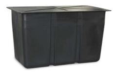
The floats, made of polyethylene, are rotationally moulded. The float can be filled with foamed polystyrene so even punctured the float is still floatable.
