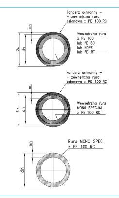
DUO SPECJAL MONO SPECJAL - monolithic pipes, singleor multi-layered with co-extrusion:
